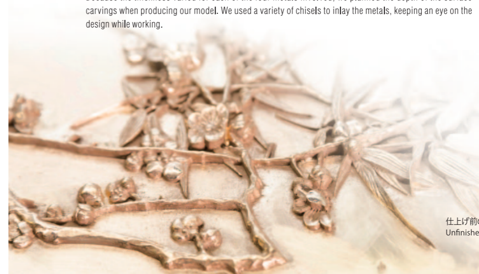
金属は、それぞれ硬さが違うため、タガネを慎重に打ち付ける。 Different chisels were carefully used to inlay the metals, taking their varying hardnesses into account.
