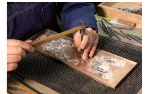
金属は、それぞれ硬さが違うため、タガネを慎重に打ち付ける。 Different chisels were carefully used to inlay the metals, taking their varying hardnesses into account.
